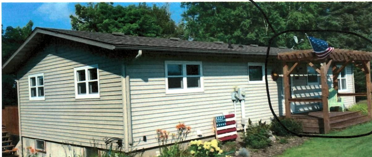
20' wide by 12' deep. It will run from just beside the entry door to the end of the kitchen window on the east side. The black area below shows the approximate size. The steps would be on the west side and railings would be placed around.
