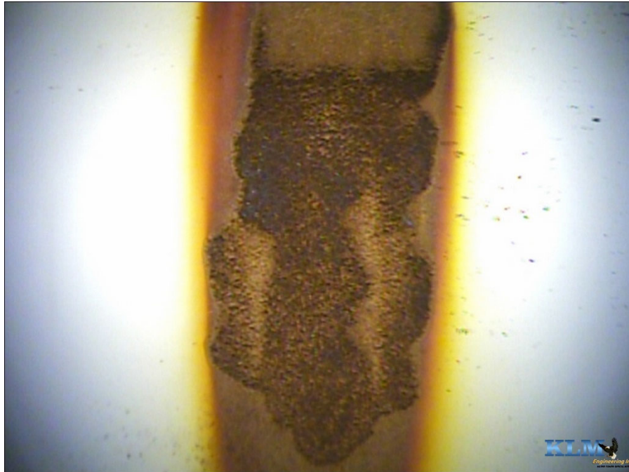
Photo No. 19 Corrosion on shell
